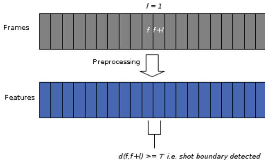
Figure 2.1: Shot Boundary Detection Concept
