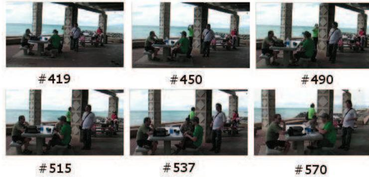
Figure 5.3: Experimental video sequence (Hawaii Flickr) with respective frame numbers. Proposed algorithm detects all these frames to be in a single video shot. Shot boundary detection using only dissolve detection, identifies the frames 419, 450, 537 & 570 to be in distinct shots, whereas frames 490 & 515 are misdetected.
