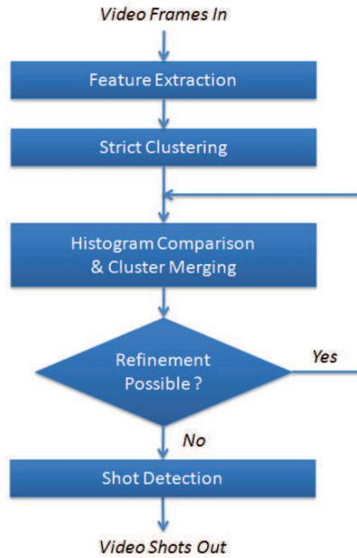
Figure 3.6: Proposed Approach for Shot Detection Using Strict Clustering
