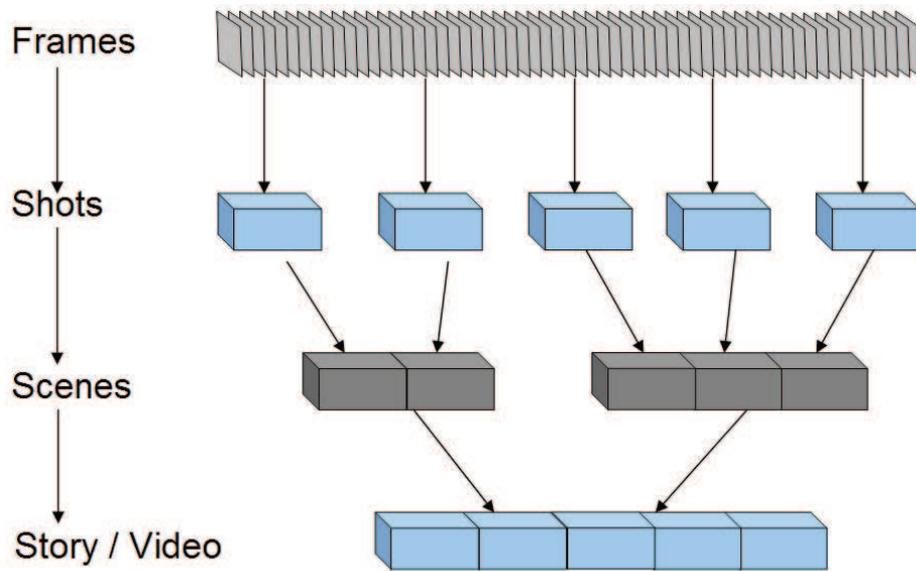
Figure 1.1: Hierarchical Structure of Video
