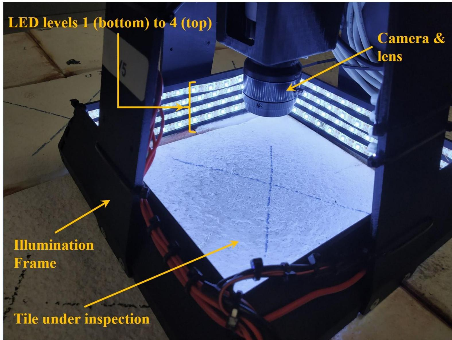
Padalkar et al., "A Versatile Crack Inspection Portable System based on Classifier Ensemble and Controlled Illumination," ICPR2020
