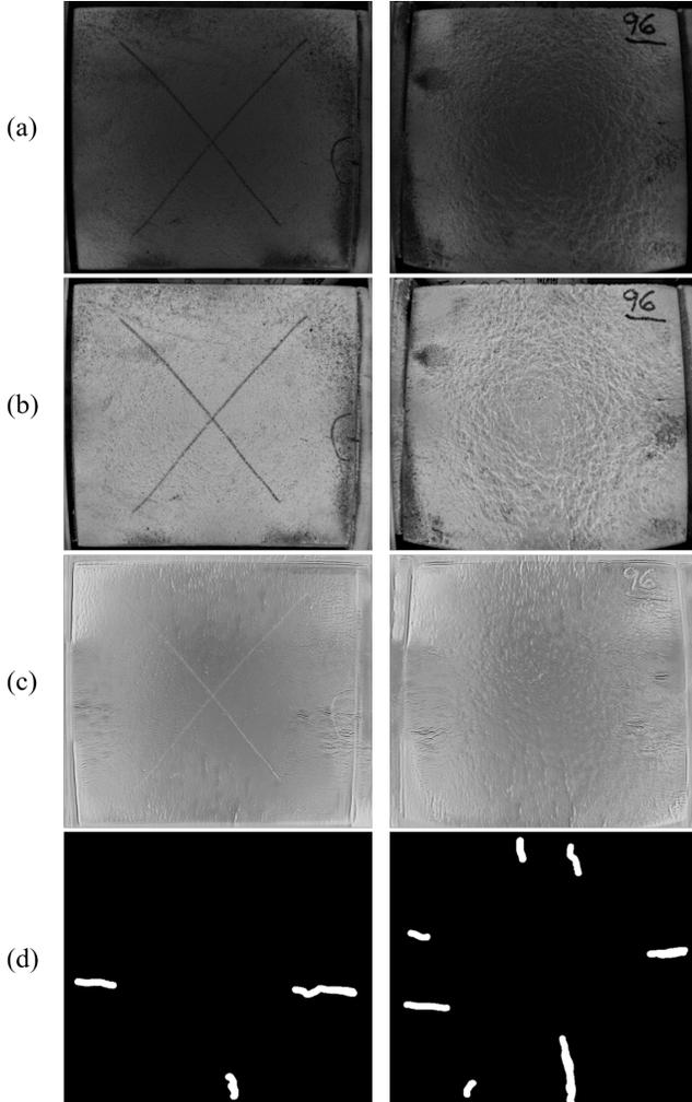
**Fig. 3.** Results: (a) Fusion with a MEF method [10], (b) initial estimate, (c) fusion with crack enhancement with our method ( $G_{A2B}$ ) and (d) crack annotations provided by experts. Notice the high contrast in (c) for regions corresponding to the crack annotations in (d). (Zoom-in for better visualization)
